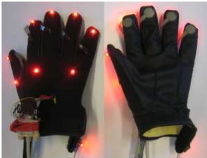
Fig. 1. Motion capture gloves with diodes and FSR tactile sensors emplacement.
